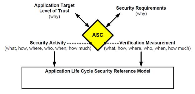
Figure 4: Components of an ASC
