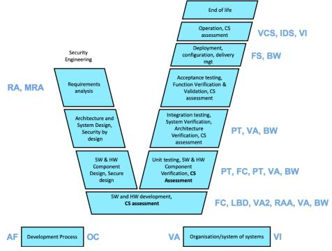
Figure 1: V-Model associated with the tools of the framework
