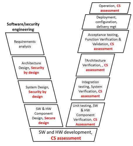
Figure 32: V-Model related to software/security engineering process
