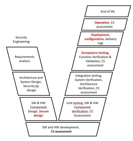
Figure 31: Firewall update - V-Model related to software/security engineering process
