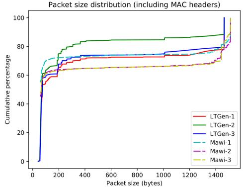
Figure 9: Packet size distributions of MAWILab and LTGen traffic
