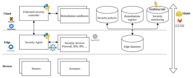
Figure 45: Vertical 1, Scenario 2 - CETIC testbed implementation and deployment view
