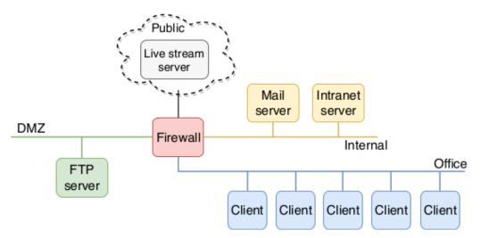
Figure 6: Network architecture hosted on the LTGen's Openstack infrastructure
