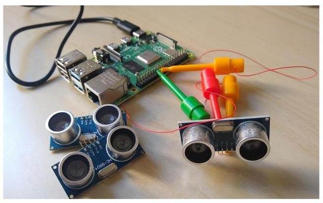
Figure 29: HW tools: Raspberry PI and ultrasounds transducer
