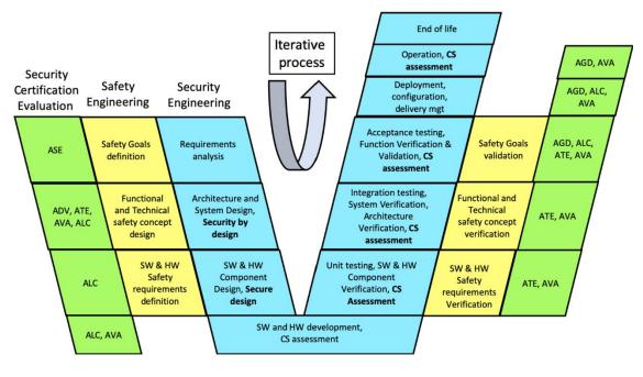
Figure 35: Different frameworks V-model appliance
